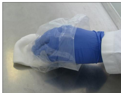
Figure 1: Wiping device gripped through a plastic bag
